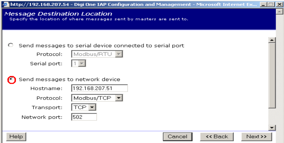
Figure 10: Network configuration of receiving device (MPiec)
